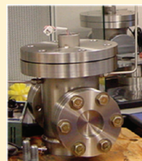
\text{CO}_2 pressure vessel for Aging/recovery experiments
